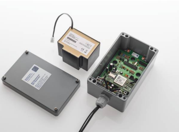
Basic unit with electronics and battery pack (plus antenna and specific sensor)
